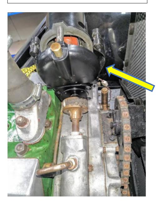
Photo 2 shows how the cars mounting strap neatly holds the ML magneto. The gasket paper is to prevent marks on the nice celluloid cover
