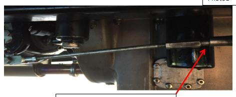
Clearance of brake rod when pedal released approx. 10mm
